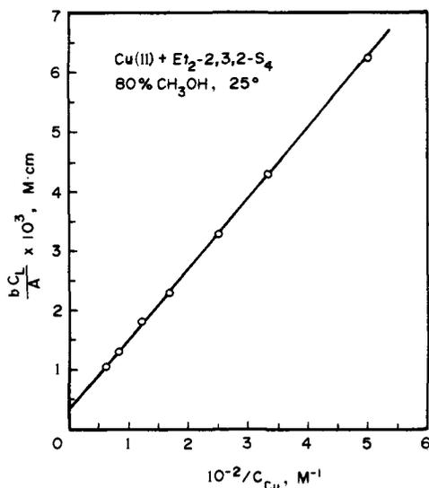
**Figure 5.** Graphical determination of the complex stability constant for the Cu(II)-Et<sub>2</sub>-2,3,2-S<sub>4</sub> system in 80% CH<sub>3</sub>OH at 25 °C, 0.10 M HClO<sub>4</sub>. The data represent absorbance measurements obtained at 414 nm and are plotted according to eq 11 to yield  $K_{CuL}$  as the ratio of intercept/slope ( $b = 10.0$  cm,  $c_1 = 5.00 \times 10^{-5}$  M).
