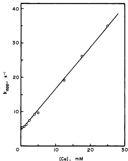
**Figure 3.** Typical plot of the collected kinetic data for a single reaction system in a single solvent composition according to eq 7 where the intercept is equal to the dissociation rate constant,  $k_d$ , and the slope yields the formation rate constant,  $k_f$ . Data shown are for the reaction of Cu(II) with 12-ane-S<sub>4</sub> in 80% CH<sub>3</sub>OH at 25 °C, 0.10 M HClO<sub>4</sub>. (The points plotted include the three values of  $k_{app}$  obtained from Figure 2.)
