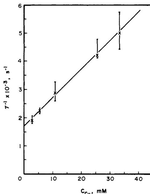
**Figure 4.** Typical temperature-jump relaxation data plotted in the form of eq 9 where the values of  $k_f$  and  $k_d$  are equal to the slope and intercept, respectively. The error bars define the range of reciprocal  $\tau$  values obtained for a minimum of five replicate measurements at each Cu(II) concentration while  $\times$  designates the median value for each data set. Data shown are for the Cu(II)-16-ane-S<sub>4</sub> system in 35% CH<sub>3</sub>OH at 25 °C, 0.10 M HClO<sub>4</sub>.
