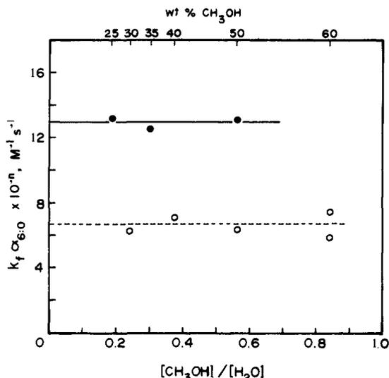
**Figure 7.** Resolution of aqueous  $k_f$  values (i.e.,  $k_{6.0}$ ) from experimental  $k_f$  data obtained in the solvent range of 25–60% methanol plotted in the form of eq 18: ○, 12-ane-S<sub>4</sub> ( $n = 3$ ); ●, 14-ane-S<sub>4</sub> ( $n = 4$ ). Increasingly positive deviations from the horizontal lines occur for  $k_f$  values as the methanol content exceeds 60% (see text and Figure 8).
