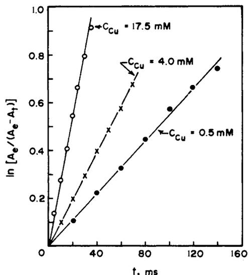
**Figure 2.** Typical stopped-flow data plotted in the form of eq 6 where the slope of each plot is equal to the respective value of  $k_{app}$ . Data shown are for the reaction of Cu(II) with 12-ane-S<sub>4</sub> in 80% CH<sub>3</sub>OH at 25 °C, 0.10 M HClO<sub>4</sub>.
